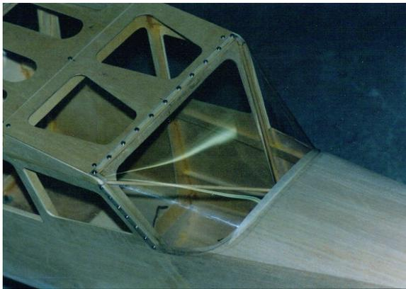
install one screw at a time. Start at the top center and work towards the outboard sides alternating sides after each screw. After the top is finished then proceed down the sides. When all the screws are in place you can remove the clamps etc. No need to apply heat to the plastic unless you see it crazing in the top corners and down the side a bit. If you see this AFTER the windshield is mounted then LIGHTLY heat with a heat gun along the craze. Keep the heat gun about 10 to 12
