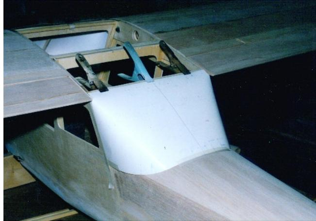
All depends on how you sanded and shaped the fuselage. Once you get the template to look good transfer this to the plastic. Repeat the procedure with the plastic. Here I put regular masking tape on the plastic to draw the centerline for reference. (Especially helps on the center bar for the windshield). After all is clamped and taped in place, drill for the mounting holes and start adding screws. Drill and
